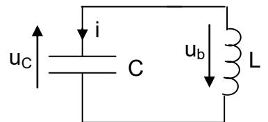
$$\text{On a } i(t) = C \frac{du_c(t)}{dt} \text{ et } \frac{di(t)}{dt} = C \frac{d^2u_c(t)}{dt^2} \Rightarrow u_b(t) = L C \frac{d^2u_c(t)}{dt^2}, \text{ on a } u_b(t) + u_c(t) = 0 \Rightarrow$$
